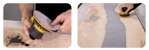
With the wood protected, it's now time to bring the resin river up to a full gloss using a polishing compound. Using a polishing machine makes the process much faster than by hand.
