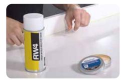
The wax will need to be pushed into the gap and any excess scraped away using a tool like a ball end wax filleting tool, then any loose wax should be removed.
