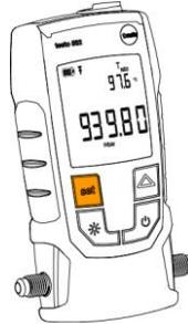
3 - Press **Δ** to set the pressure unit required.
