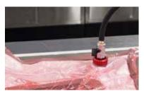
Good practice is to perform a drop test which will highlight any leaks within the system. Leaks in the system will not only compromise the final part but can also damage your vacuum pump, so they are best to be avoided if possible. Without a gauge, the drop test
