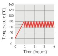
they are set too. Typically, the temperature inside the oven will cycle a few degrees above and below the set temperature as the thermostat cycles on and off. This creates a less than ideal sawtooth profile, as seen in the graph opposite. In the example shown, the temperature in the oven is set to 70°C but inside the oven cycles between 60°C
