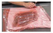
The part can now be placed in a vacuum bag in a similar way to when doing the debulk. The main difference being the use of an unperforated release film which will preserve the resin to fibre ratio, keeping it balanced throughout the cure. Placing breather on the
