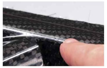
However, due to the inherent inaccuracy of curing in a conventional thermostatically controlled oven, components cured in this way may exhibit some minor pin-holes under close inspection.
