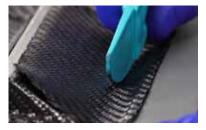
The prepreg patterns can then be placed into the mould, generally the paper side of the material goes face down onto the mould. Leaving the plastic backing on for the initial placement stabilises the material to prevent distortion, keeping the surface tack free
