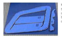
Masking tape templates are then transferred to a sheet of card and slightly oversized by ~5mm to allow for some overlap.
