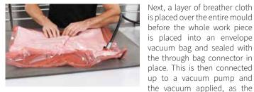
vacuum is drawn the bag can be slid into position to ensure that there is no bridging. Full vacuum should be held for 20 minutes to ensure that the material is fully pressed onto the surface.
