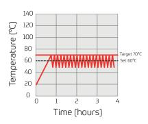
From this test we know that our oven peaks roughly 10°C higher than the set temperature, so in order for us to cure the prepreg with the peak temperature not exceeding the target temperature, we will need to set the oven temperature 10°C lower than the target temperature.
