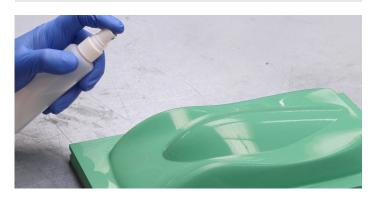
Depending on the level of gloss required, once the machined board has been finished to the required standard it can either be coated directly with a suitable chemical release agent (such as **Easy-Lease**) or it can be first sealed using a specialist board sealer before applying release agent.
